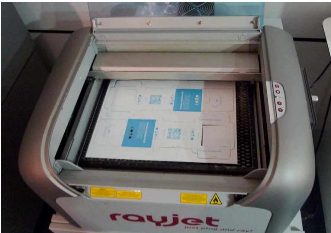
Figure 44 - First tests with the laser cutter were not so successful as it was difficult to match and align the scales with the printer and the laser cutter.
