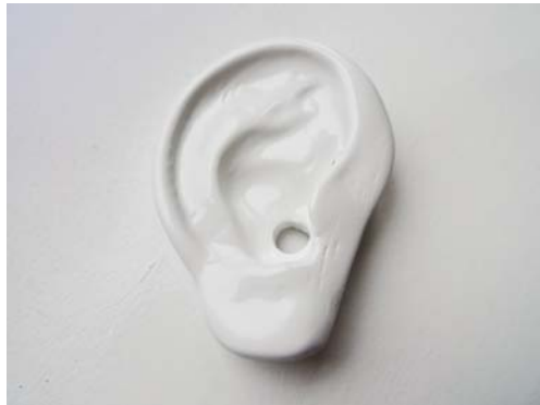
Figure 35 - Halfway through priming the surface of the ear to fill in the small grooves and build lines from the rapid prototyping printer.
