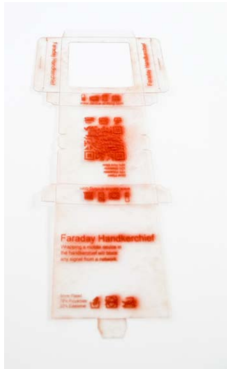
Figure 50 - Clear sheet after laser engraving before it is cleaned and assembled.
