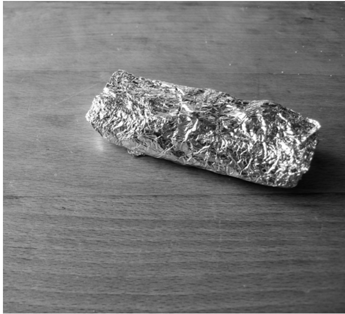
Figure 64 - First test of faraday cage for the mobile phone. It worked wrapping it in tin foil which led me to try it with conductive fabric.
