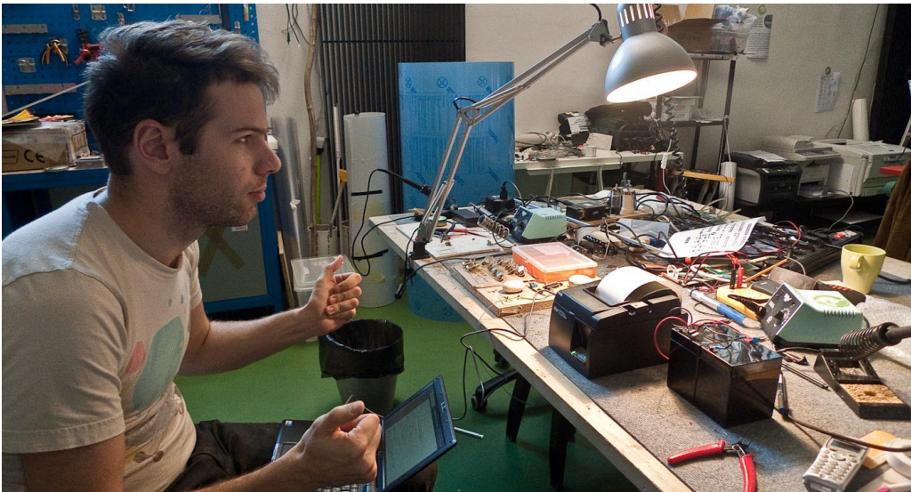
Figure 31. Newsleak disassembled: the Netbook, sending output to the battery- powered thermal printer
